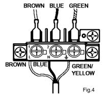
If the cable has to be threaded through small apertures in cabinets etc., it may be disconnected from the appliance, then re-connected to as shown in Fig.4.
